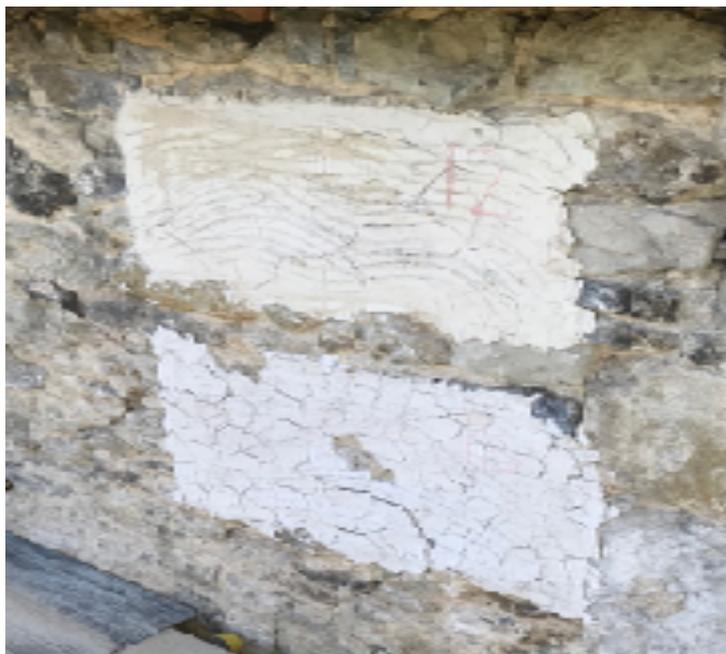
**Plate 4: Lime rich mortar samples that were subject to failure at The Church of St Mary the Virgin, Oxted**
